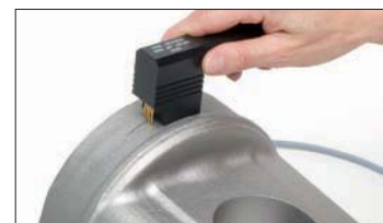
Crack depth measurement of an inclined crack after angle determination
